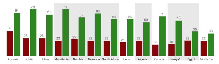
1. Solar power potential (in kWh/kWp) and wind power potential at 100m height above ground (m/s)
